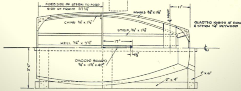
HULL TO BE BUILT UPSIDE DOWN ON THIS BASE WHICH CAN BE USED ANY NUMBER OF TIMES. BUILD BASE TRUE AND SQUARE.
